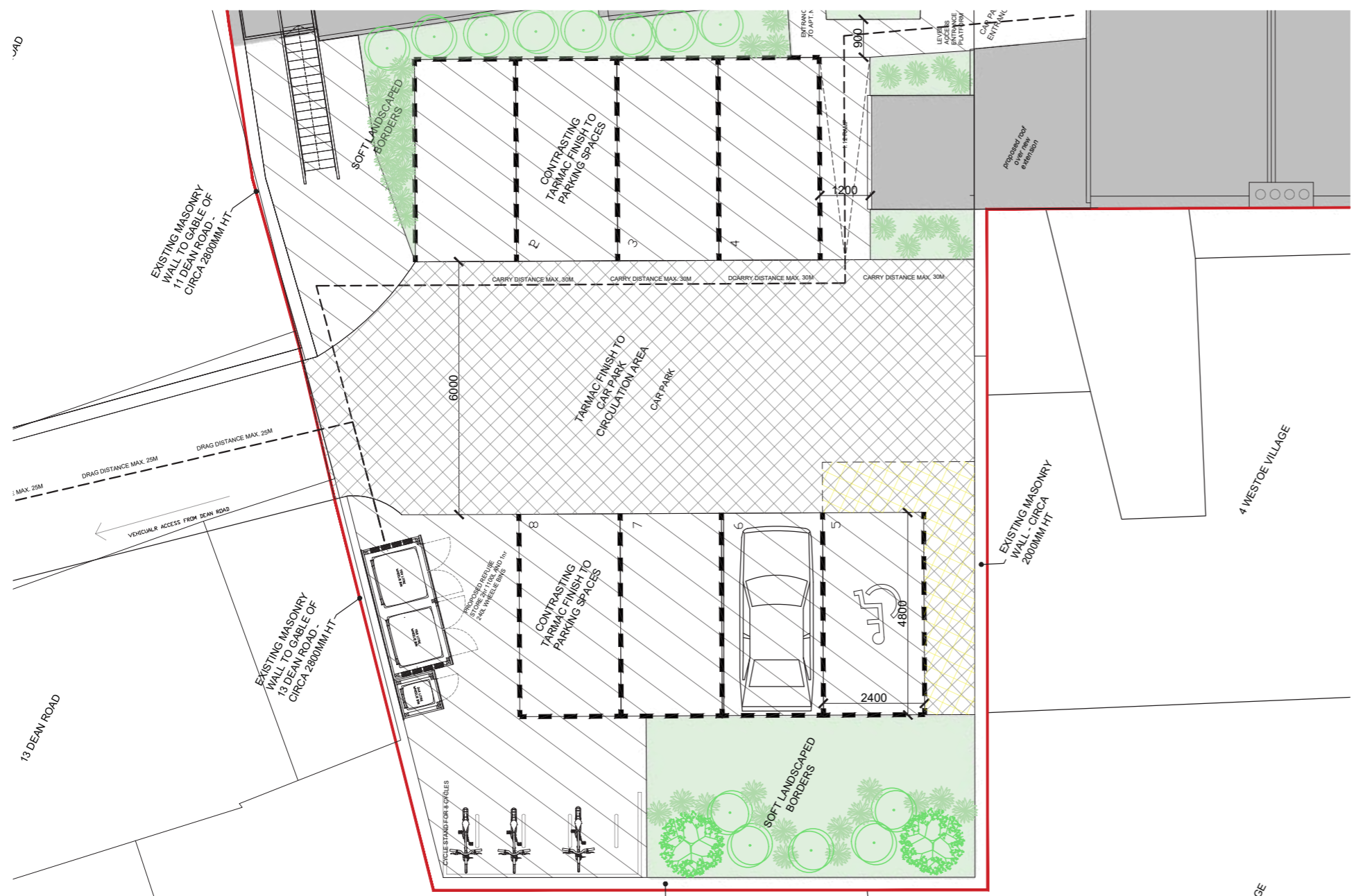
PROPOSED CAR PARK INCLUDING ACCESSIBLE BAY AND CYCLE STORE (RES736-BHA-00-ZZ-DR-A-1201 PROPOSED SITE LAYOUT)
